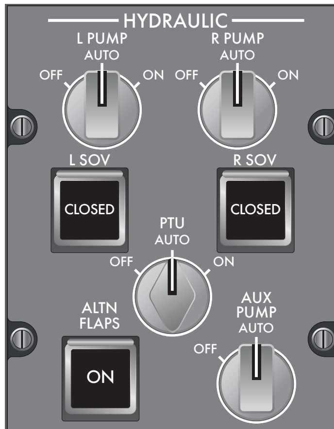
Hydraulic Control Panel
