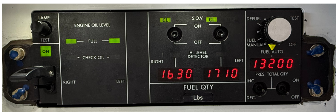
Remote Oil / Fuel Panel
